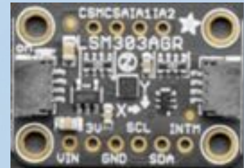
Accelerometer Magnetometer ( measures magnetic field and acceleration )
