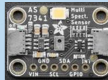
Light Spectrum Analyzer (measures multiple colors and ranges of light)
