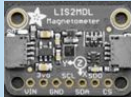
Magnetometer ( measures magnetic field )
