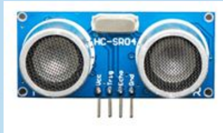
Ultrasonic Distance Sensor (measures short distances using ultrasonic sound waves)
