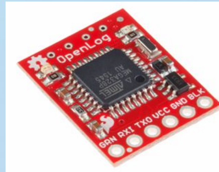
Data Logger (has a microSD card soldered on)
