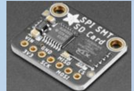
Adafruit SPI Flash SD Card (has a microSD card soldered on)
