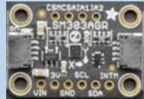
Accelerometer Magnetometer ( measures magnetic field and acceleration )
