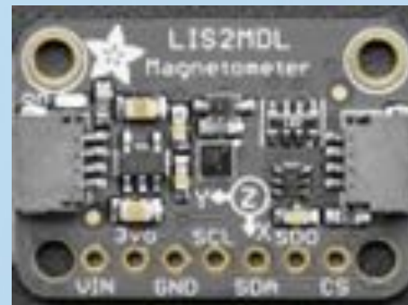
Magnetometer ( measures magnetic field )
