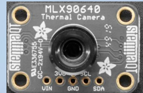
Adafruit Infrared Thermal Camera (takes "images" showing a grid of the temperatures it sees)
