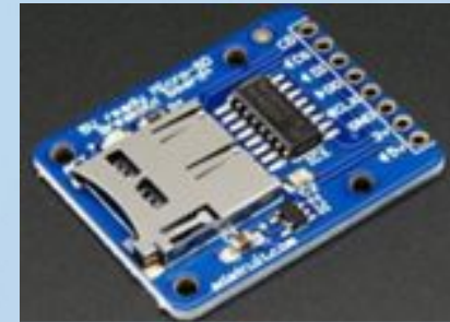
MicroSD Breakout Board (has a slot to hold a microSD card)
