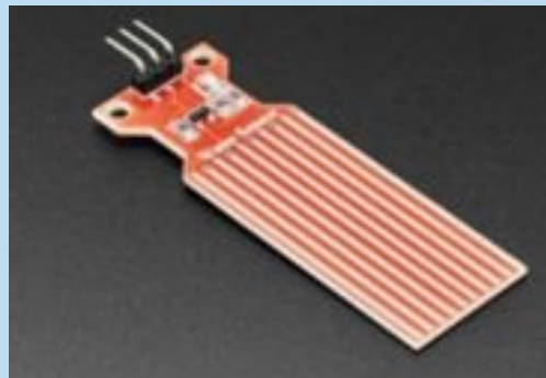
Water Sensor (detects the presence of water)
