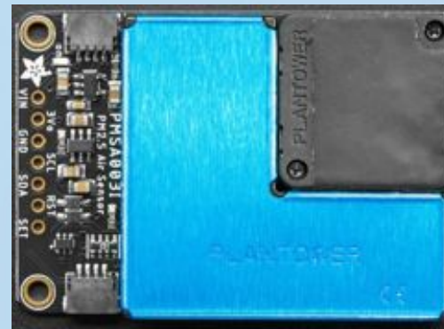
Air Quality Breakout Sensor (measures particles in the air such as dust, pollen, or smoke)
