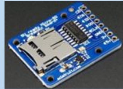
MicroSD Breakout Board (has a slot to hold a microSD card)
