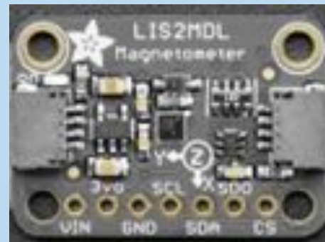
Magnetometer (measures magnetic field)
