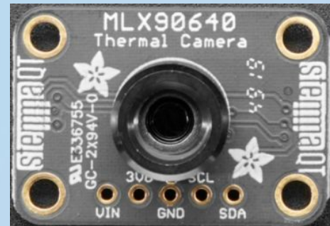
Adafruit Infrared Thermal Camera (takes "images" showing a grid of the temperatures it sees)
