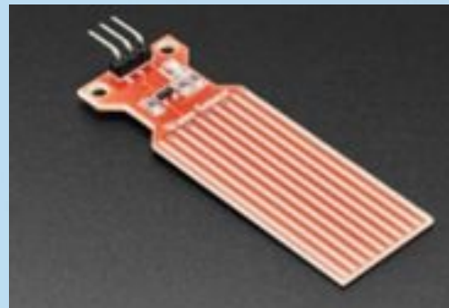
Water Sensor (detects the presence of water)
