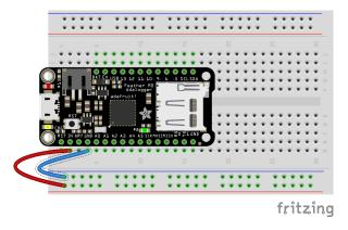
Step 2: Connect the sensor on the board as shown with the front grid facing the bottom of the breadboard and connect a red wire to the 1stpin on the left of the sensor and the red power rail at the bottom. Then connect a bluewire to the 3rd pin from the left to the blue ground rail on the bottom of the breadboard.
