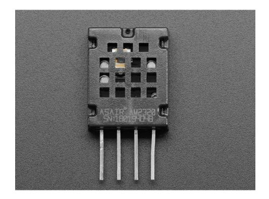
From left to right: VDD (voltage), SDA (serial data), GND (ground), SCL (serial clock)
