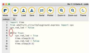
5. To correct the code, we can change the Capitalized "W" in "While" to a lowercase w. Press the "Save" button in the Mu Editor and your code will begin running and your LED light on the microcontroller will begin blinking.
