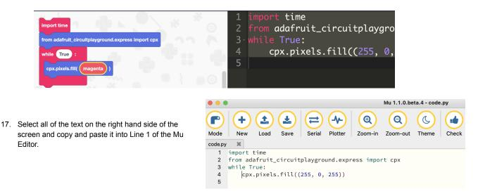
18. Before pressing save, ensure that there is no current code running on the microcontroller by clicking the "Serial" button at the top of the Mu Editor.
