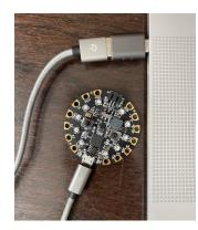
Note that your microcontroller may have been pre-programmed and may start lighting up automatically. If it does, press the tiny "reset" button in the middle of your microcontroller board. If it doesn't reset, that's okay! We will reset it later in this lesson.
