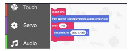
The neopixels are full color, RGB LED lights. This means we can manually alter the red, blue, and green colors within each pixel using numbers between 0-255 with the following code format:
