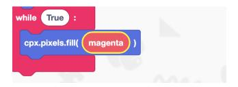
16. Take note of how the native CircuitPython code is building on the right hand of the screen in EduBlocks. We are now going to open our Mu Editor and copy and paste the native code into Mu and upload it to our Circuit Playground microcontroller.
