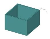
Minimum recommended wall thickness for your model is 1.5 mm.
