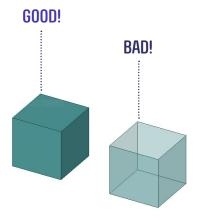
Your 3D model should be solid geometry. For example, the model on the right has no top surface and zero wall thickness. This is not 3D printable for the prize. Most models in Tinkercad or other CAD programs make solid models, so you're probably fine! But if in doubt, upload your STL file to Meshmixer and check.
