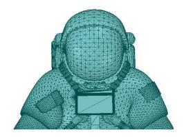
For example, this mesh is complex, but is under 20MB if exported properly. Chord Tolerance or Angular Control can be modified in some advanced 3D software packages to change the resolution of your STL file export. Otherwise, in Meshmixer you can upload your STL file and re-export it using the STL Binary Format to reduce file size.
